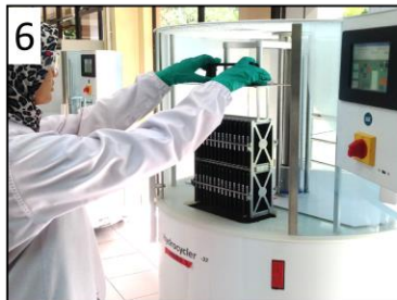
6 DNA amplification ❖ Water-based thermal cycler
